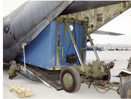
Dolly Set Loaded into C130 Aircraft with 8-ft. x 20ft ISO Container.
