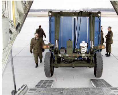
Dolly Set Loaded into C130 Aircraft with 8-ft. x 20ft ISO Container.
