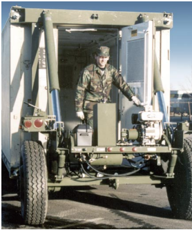
Rear Dolly Permits Full Opening of 3-4 ft Wide Access Doors.
