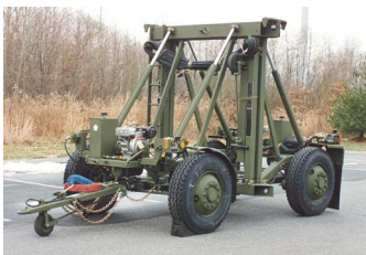
Dolly Set in 4-Wheel Mode (Unloaded)
