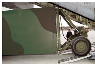
M1022-A1 Dolly Set Loading Shelter onto C130 Aircraft
